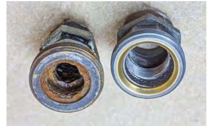
Contaminants build up when laminar boundary is intact but when collapsed, they're removed by sheer force of the water.
