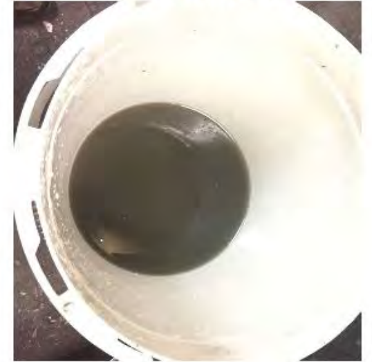
PARTICULATE REMOVED FROM CT BASIN WATER WITH ELECTROCELL
